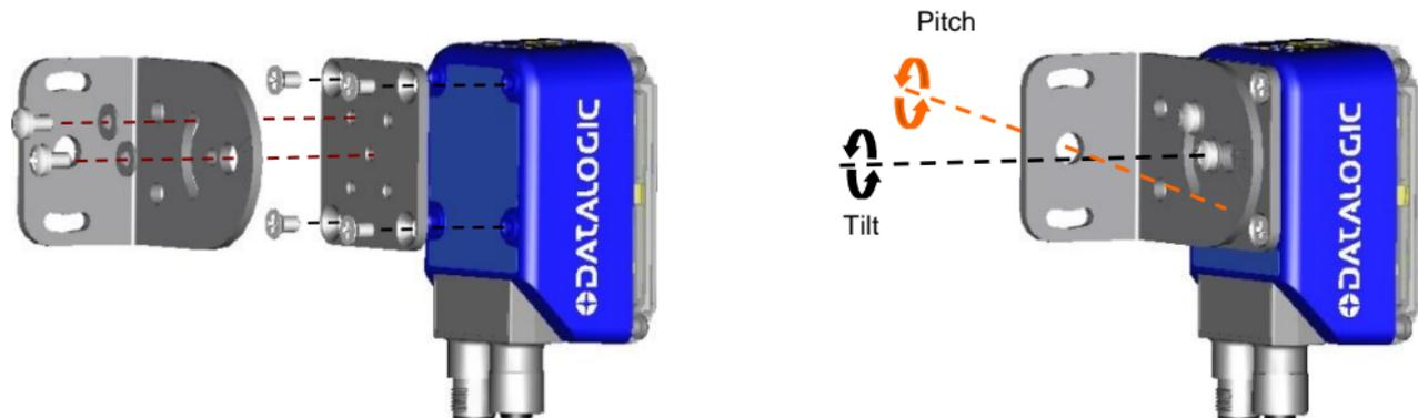
Figure 2 –Positioning with Mounting Bracket
