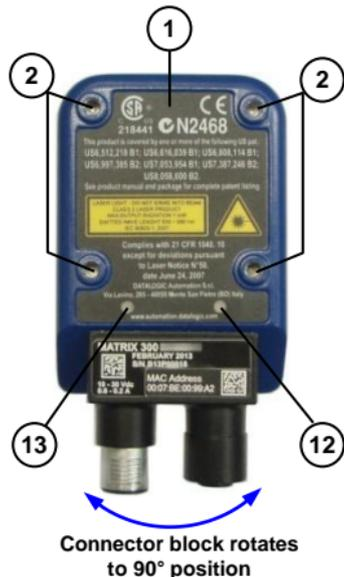
Connector block rotates
